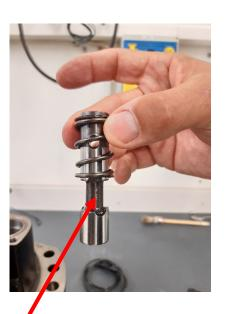
Valve with spring - correct position
